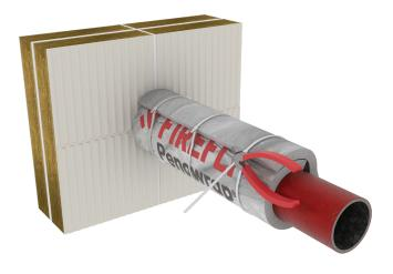
Install a fillet or bead of FIREFLYMastic with the dimensions given in the specific Warringtonfire Report ID if required. In some instances, a second layer of FIREFLY Penowrap is required.
