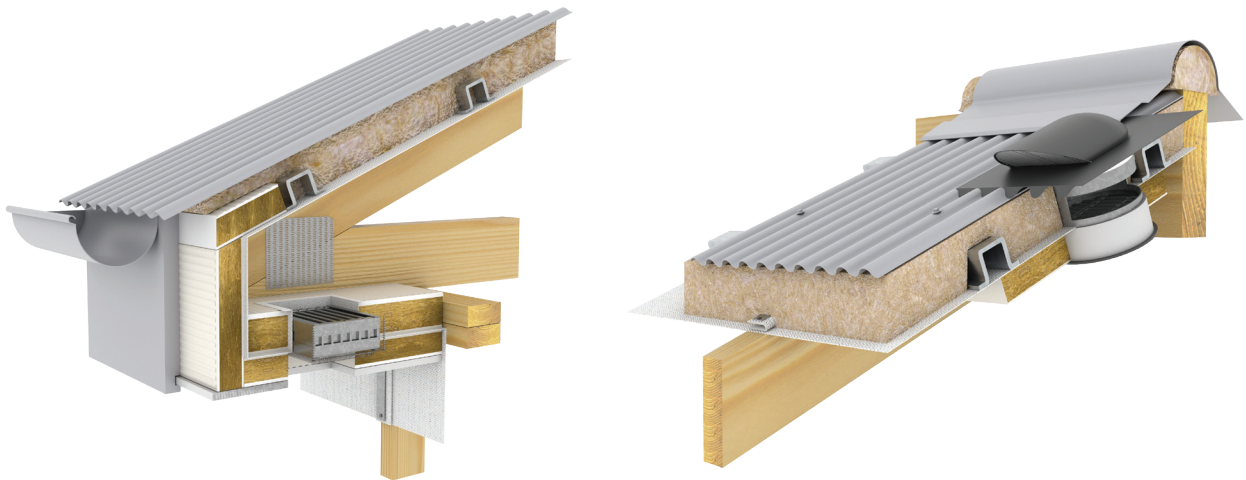
Illustrations showing protective vents installed at eaves and roof of FIREFLY BAL-FZ Roof System
