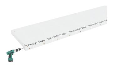
Fold the overlap and secure using a minimum 32mm 4.2g pan/button head self-drilling screws.
