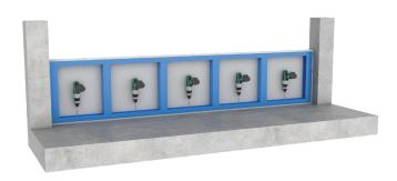
Secure the bottom track into the concrete using minimum 40mm M6 masonry screws/anchors at nominal 600mm centers and 50mm from both ends.
