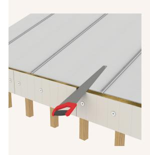
Trim off the excess FIREFLYBatt FZ, creating a raked finish flush to the angle of the roof using a wood saw.
