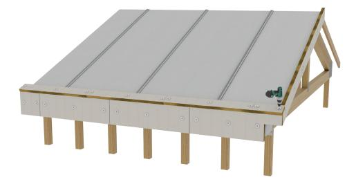
If a gable is present, install the FIREFLYBatt FZ to cover the barge end, and the ends of the battens in Steps 13 & 23. Extend by 42mm for a **sheet metal roof**.
