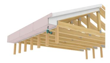
at nominally 300mm centres through the timber framing or steel angles. Seal all joints with FIREFLYMastic.
