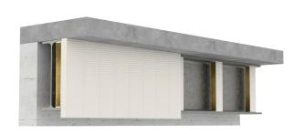
Cut a batt to a width corresponding with distance between the slab underside and bottom flange, adding 50 mm for the bottom flange overlap.
