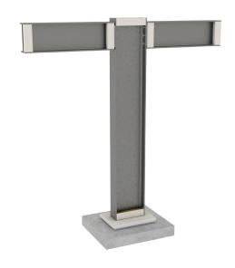
Repeate Steps 3 and 4 for the steel beam ie. install end noggings. Also install noggings at the intersection joint.
