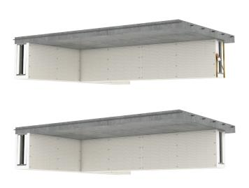
Apply extra FIREFLYMastic BG on all the joints / corners / edges, ensuring that there are no visible cracks or exposed green edges of the batts as seen from outside.
