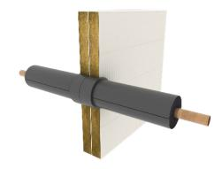
V120 - Up to 200 mm copper pipe with minimum wall thickness 3 mm and 75 mm thick stone wool foil faced continuous lagging. FRL -/180/180
