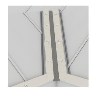
Seal the valley gutter's upper edge to the adjacent top-hat with FIREFLY Silicone.
