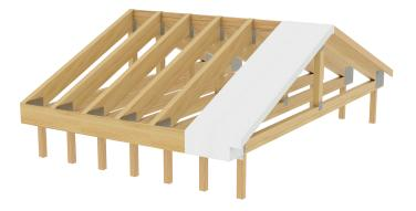
Note: The Plus 60 blanket is 1300 mm wide allowing for most efficient use on 600 mm truss or rafter spacing. For details on alternative frame spacing, refer to Appendix A.
