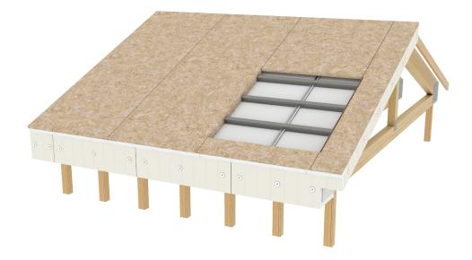
The fascia is fastened over the FIREFLYBatt FZ with either fibre cement or plasterboard through to the truss ends; with fasteners and brackets accounting for the additional thickness from the protection system.
