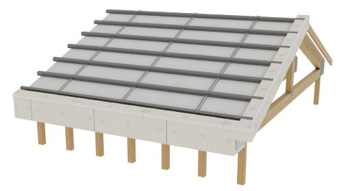
For gable sections where the top-hat battens interface with 25mm wide, vertically oriented FIREFLYBatt FZ install setions of FIREFLYBatt FZ between top-hats, butting up to the batten and vertical FIREFLYBatt FZ on the barge, using
