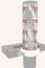
Beyond 40 mm OD steel pipes up to 300 mm OD can achieve FRLs up to -/120/120. Only increase the fillet size to 50 mm
