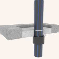
The largest FIREFLY FRF collar, FRF 150, can provide an FRL of -/120/120 to a 160 mm HDPE pipe when installed under FIREFLY-Mortar substrate
