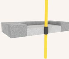
FIREFLYMastic HP around Gas PEX pipes in FIREFLY-Mortar achieves an FRL of -/120/120
