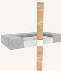
Bare copper and ferrous pipes up to 210 mm OD installed in FIREFLYMortar can achieve an FRL of -/120/- using only FIREFLYMastic
