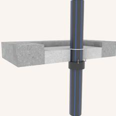
100 mm HDPE pipes with a maximum wall thickness of 7 mm achieves an FRL of -/120/120 with FIREFLY FRF 100 collar under FIREFLY-Mortar substrate
