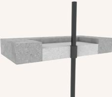
FIREFLYMastic HP around PEX pipes in FIREFLYMortar can be installed using bubble wrap or a backing rod
