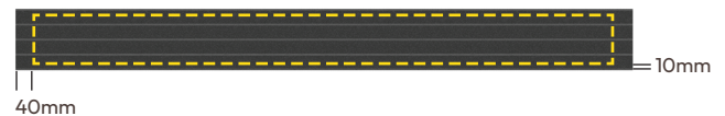
Figure 4 - Penetration allowable zone for FIREFLY FR Block within apertures 1000 mm x 100 mm
