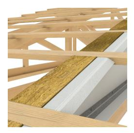
**Note:** For un-sarked roofs, it is recommended to pack tightly the area between the top chord and the roof covering, between the roof battens, with FIREFLY Party Wall Batt, compressed by 15%. Ensure the barrier overlap is tightly sealed to prevent the passage of smoke.
