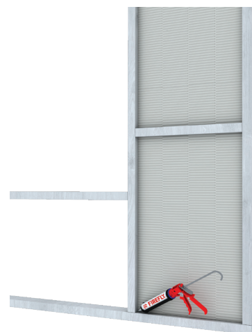
Joint sealing RetroBatt 60 to frame joint
