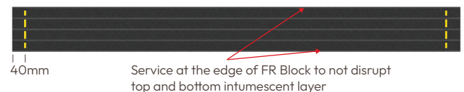
Figure 4 – Penetration allowable zone for FR Multi-Service Block within apertures 1000 mm x 100 mm
